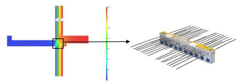
Energy flow diagram produced for a balcony to internal floor/external wall junction, produced from a Psivalue calculation. Example Schock Isokorb thermal break was tested to mitigate this thermal bridge.
