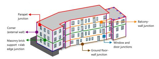
*Example of the location of thermal bridge junctions. Different colours indicate the different types of thermal bridge that exist in this scheme. Typically a Psi value would be calculated for each of these junctions.*
