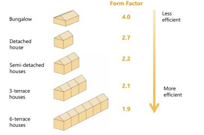
**2. Simplify form** by reducing overly articulated shapes such as stepped roofs, stepped facades, overhangs, roof terraces and inset balconies. By simplifying the building form, the exposed surface area is reduced, complicated architectural details are mitigated, and cost is brought down.
