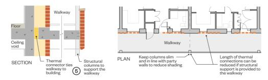
Diagram illustrating how to design out thermal bridges on access walkways. Source: Passivhaus easi-guide
